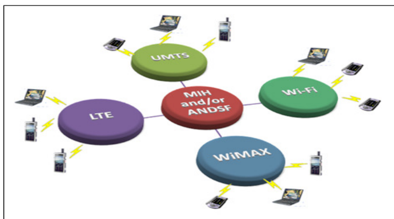
Figure 1: Various Radio Access Technologies (RATs) integration supported by MIH /ANDSF
