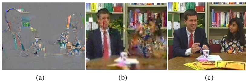
Figure 8. Paris sequence (a) using AODV with random scheduling (b) using AOMDV with random scheduling (c) using AOMDV with the proposed scheduling
