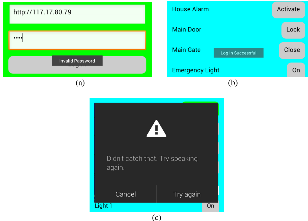
Figure 9. Screenshots of the proposed smart home app: (a) when invalid password is entered (b) when login is successful (c) when no voice command is captured.
