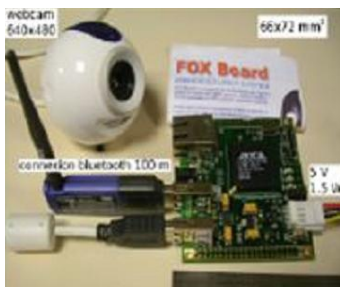
Figure 7. Sensor implemented using the fox board.
