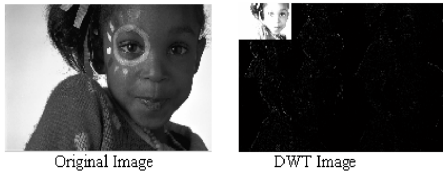
Figure. 2. Original Image and Pyramidal Decomposition after DWT application for level=2
