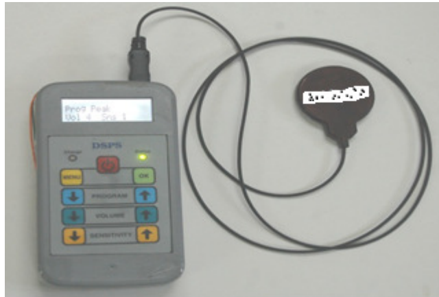
Fig 4: Prototype to Product Model of FPGA based Speech Processing System with RF Transmitting Coil.
