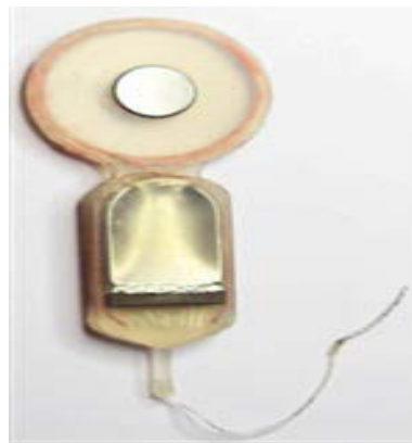
Fig 5: Prototype to Product Model of Implantable Receiver Stimulator with RF Receiving Coil.
