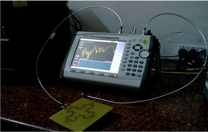
Figure 11. Laboratory setup for measurement of return loss and VSWR.
