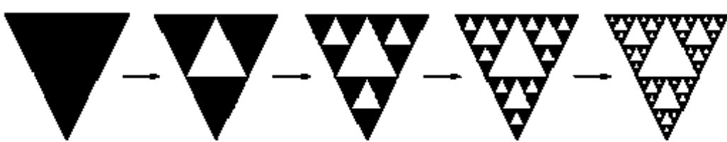
Figure 5. First four iteration of Sierpinski Seive antenna [10].
